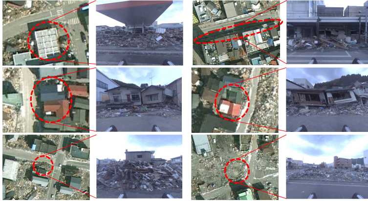
Fig. 2. Example aerial and street-view images. There are many cases in which aerial images and street-view images give complementary information about the land surface condition. For example, the areas covered by the building roof (the top and second row), stacked objects (the bottom row) are best viewed from the street.
